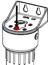
4. Press the red button at the top of the filter unit to exhaust the pressure in the system. It will not be possible to unscrew the filter canister if this operation is not carried out.
