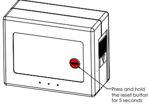
11. Press and hold the reset button on the filter change indicator module for 5 seconds. The LED light on the tap will glow red, followed by yellow, and then the module will emit an audible beep. The filter change indicator is now reset.
