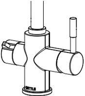
4. Turn on the boiling water again to release the pressure in the system. **IMPORTANT NOTE:** If you do not follow this step the pressure trapped in the system will make it impossible to unlock the filter housing sump from the head.
