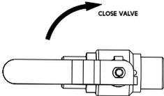
3. Shut off the water supply to the filter using the adjacent stop-valve.
