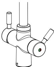
9. Operate the system and run the boiling water for a few moments until the water runs clear. Run the boiling water for a moment to release any trapped air.
