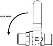
8. Turn the water supply 'on' and check the system carefully for leaks.
