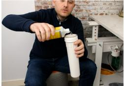
Carefully pour all of the cleaning fluid into the sump.
