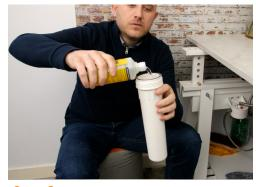
Carefully pour all of the cleaning fluid into the sump.
